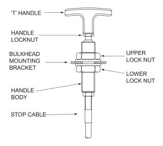
**Note:** On larger spindle valves it requires significant force to move the valve to the fully closed position using the RTD-100 handle whilst the engine is not running. This is a design feature and adjustment is not necessary. When the engine is running, manual shut down will be achieved satisfactorily using considerably less force to operate handle RTD-100.
